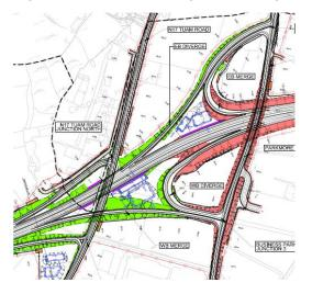
**Recommendation:** The Designers should assess whether the diverge for the N17 and merge for the mainline from Parkmore Link Road are required as there appears to be an alternative route within the proposed design for each of these movements. If a merge and diverge was removed from the design these issues would not arise. Please also refer to comment 3.5.
