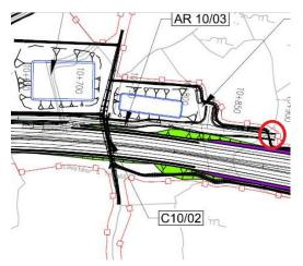
**Recommendation:** The Designer should assess how an over height vehicle will reach the local road network having been directed from the mainline at this location. Measures should be put in place to make the required movements as simple as possible.
