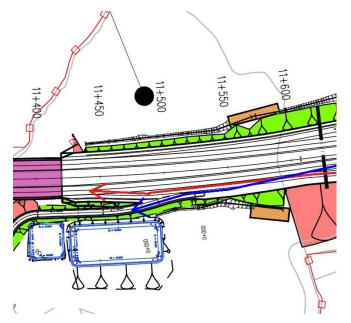
**Recommendation:** The Designer should investigate widening the tunnel to include a hardshoulder or to extend the merge/diverge lanes through it. This would simplify the provision of signage on the eastbound direction and will reduce the potential for the collision types outlined.
