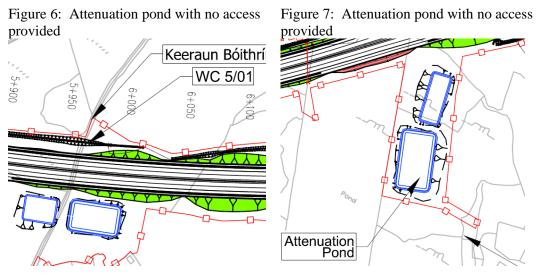
**Recommendation:** The Designer should ensure that all attenuation ponds are provided with an access either from the proposed scheme or the existing adjacent road network.
