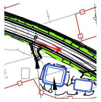
**Recommendation:** The Designer should ensure that they have allowed sufficient land take to provide the required visibility at all road junctions. The Designer should also demonstrate that sufficient visibility is provided by the preparation of the appropriate drawings.
